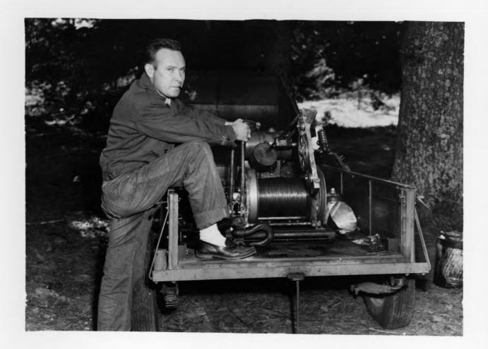
View of Halliburton Reel in Operation for Testing Diamond Drill Hole Deviation
