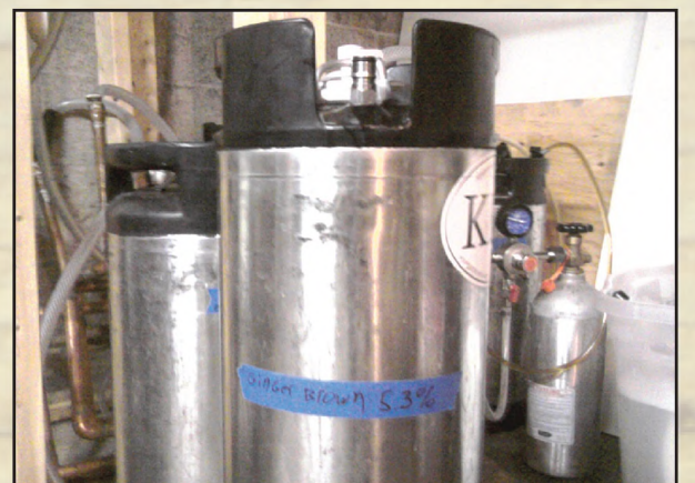
Cornelius kegs, typically three, five or ten gallons, can keep beer fresh for up to six months if stored properly.
