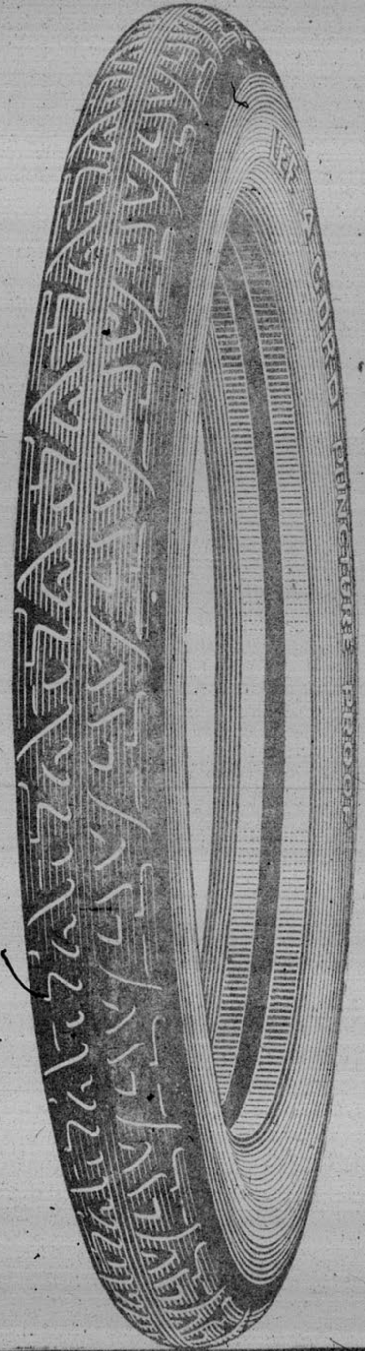
Three layers of case-hardened steel discs, individually imbedded in pure rubber, built into every Lee Puncture-proof Cord tire protect inner-tube and carcass, and enable it to live up to its name.
